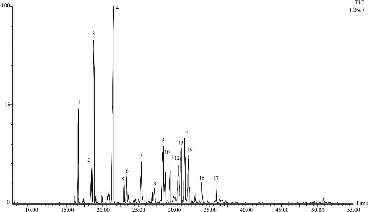
Figure 1. GC-MS Chromatogram for *Vernonia amygdalina* essential oil.
